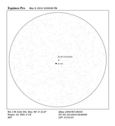
The second image below is what you would see with a Newtonian telescope at 56 power. This type of scope reverses north and south, and also east and west, due to the path light takes inside the instrument. Binoculars, as shown above, show the same "normal" relationship that the naked eye sees.
